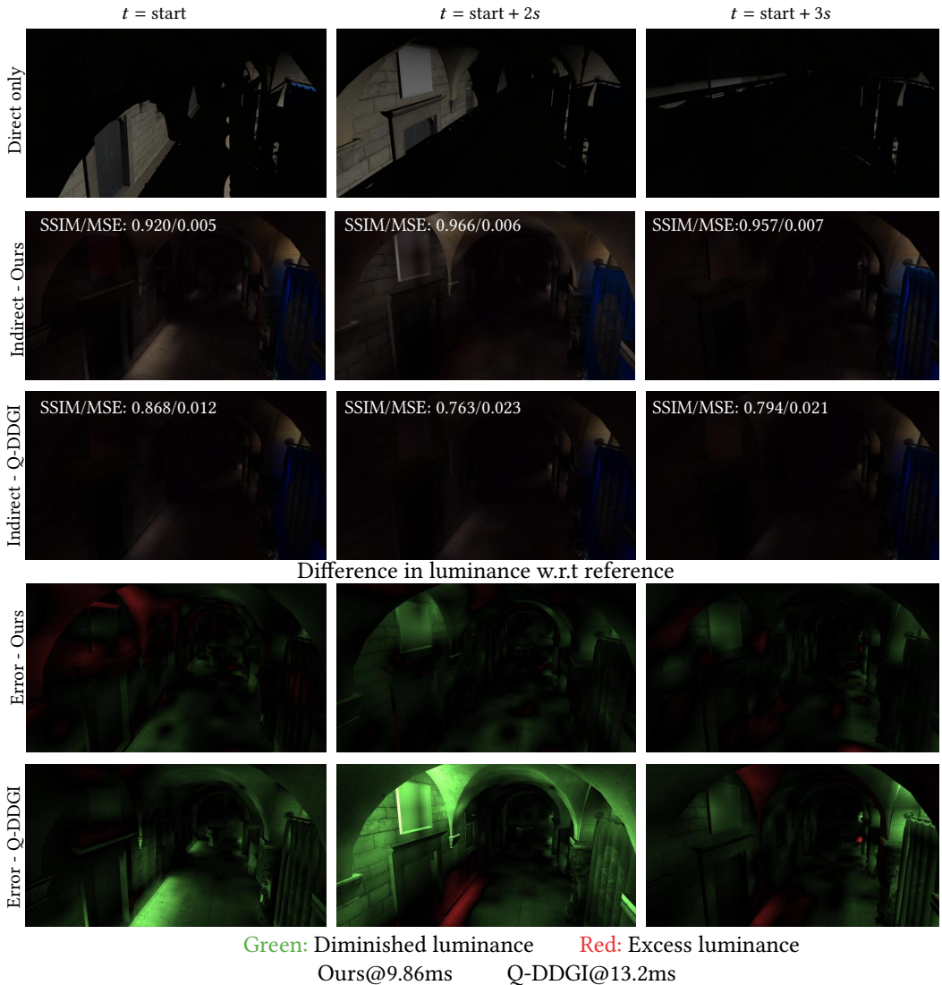
Fig. 9. Figure comparing the convergence of our technique under dynamic lighting controlled by the direct component shown in the first row. The last two rows measure the difference in luminance w.r.t reference and highlight the error in red and green color.
